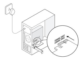
5. Locate an available **F\_USB** connector and carefully plug the Bluetooth USB cable into it.
