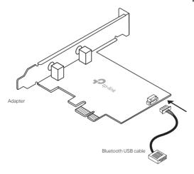
4. Locate an available PCIE X1 slot and carefully insert the adapter.
